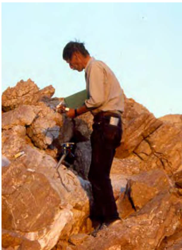
5-Jean just achieved to drill a core for paleomagnetic studies in the lower Triassic limestone of Wadi Musjah (January 1995, Oman)
