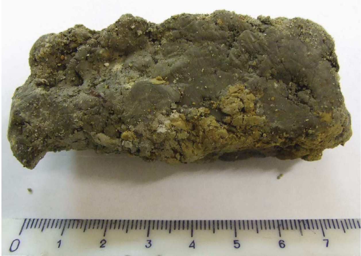
Figure 1.12. Red-brown (rust) layer in a base of transitional layer.
