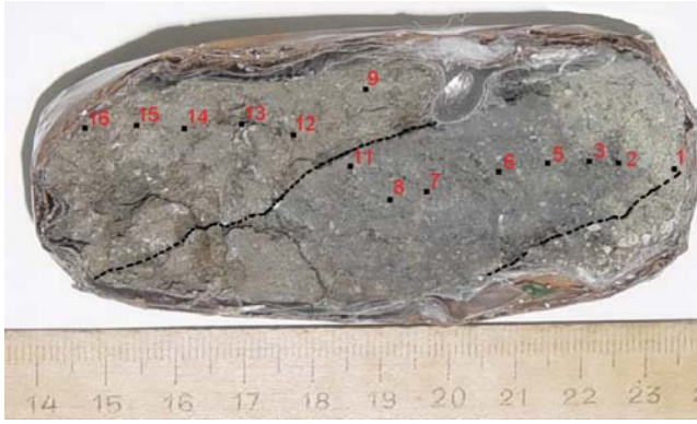
Figure 5.24. Enumerated are interlayers fragments from which were taken for the study of magnetic properties. The hatched line shows the top of the Gams-2A boundary bed. The visible thickness of the bed is 36 mm.
