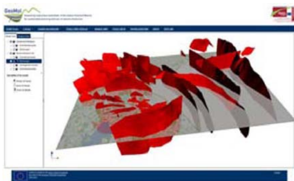
Figure 2 – GeoMol's web-based 3D viewer portraying the fault network of two 3D geological models of the cross-border Upper Bavaria – Upper Austria area (screen dump of the beta version). The two 3D models displayed are stored separately at the legally mandated geological survey organizations and merged on-the-fly via the web (from Diepolder & GeoMol Team 2014).
