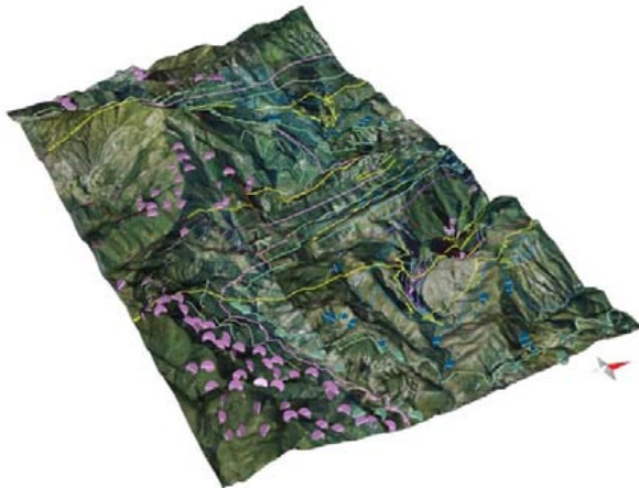
Figure 3 – Single Move model composed from GIS raster, outcrop vector, and GST database sources
