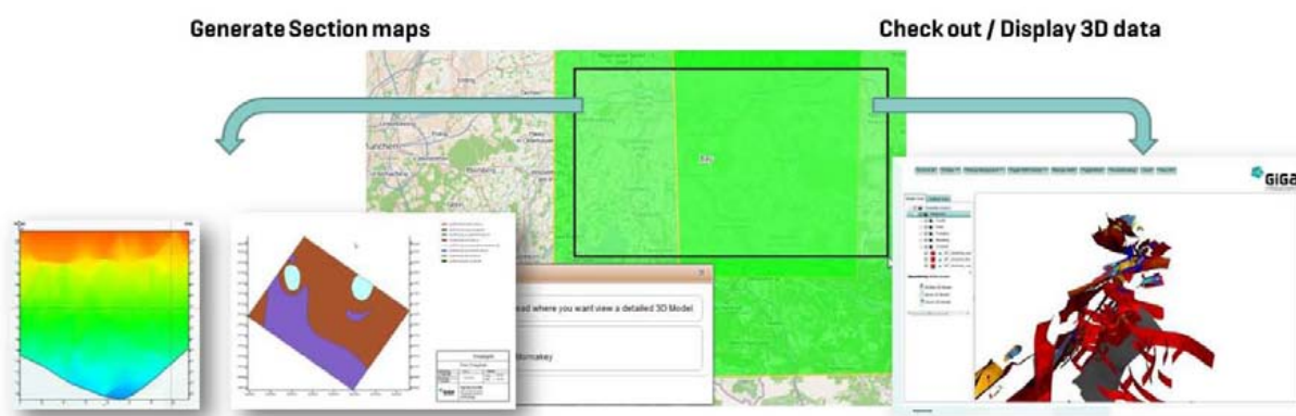
Figure 2 – 3D boxes containing subsets of the geomodel of the subsurface can be selected using the 2D web mapping application (center), and then appropriately and efficiently visualized. A modeled property like temperature can be displayed in vertical cross sections slicing the 3D box, and a geological map at a given depth can be displayed as a horizontal cross section within the box (left). The portion of the 3D geomodel within the box can be visualized as interactive WebGL scene (right) and instructively inspected without any additional visualization software.
