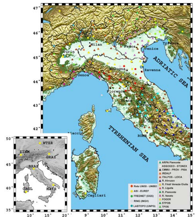
Figure 1 – Distribution of the GNSS permanent stations analyzed in this study. The commercial and scientific networks are respectively represented by triangle and circle. The institutions and companies that manage the sites are identified with different colours. The positions of the 5 IGS sites used to align the daily solutions to the ITRF2005 reference frame are shown in the inset.
