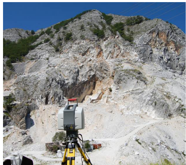
Figure 1 – Terrestrial laser scanner operating at the Apuan Alps Marble District (Carrara, Italy).
