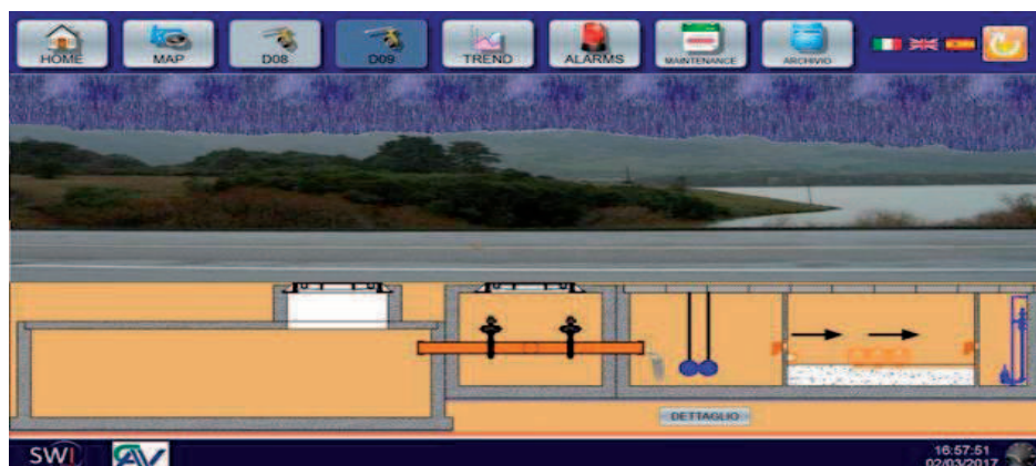
Figure 3. Normal operation of the Stormfilter® and Swerm® in wet conditions from the supervision system
