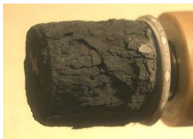
Figure 65: Corrosion test sample from Soultz (carbon steel exposed for 10 days in non-alkaline brine with 0.02 m CO 2 at 200 °C (Muller et al., 2007).
