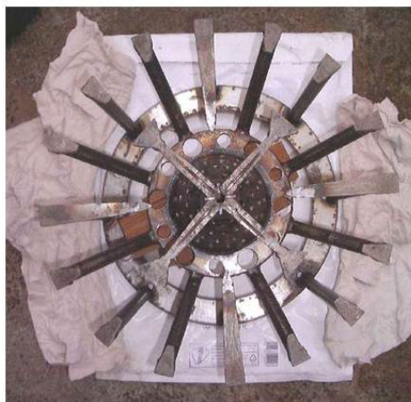
Figure 62: Picture of electro-pulse drilling bits (Bommer, 2012).
