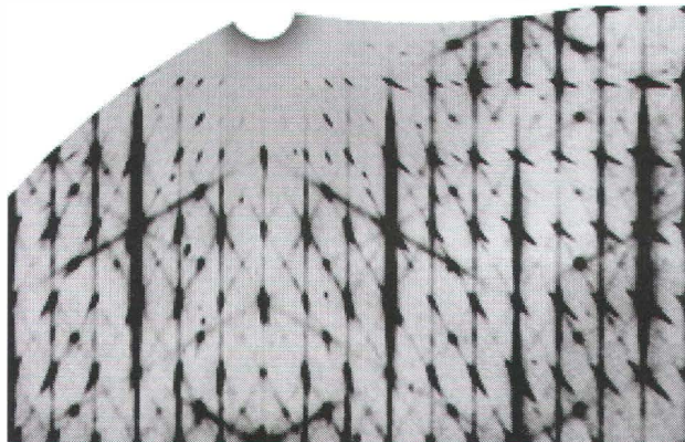
Figure 3: Reciprocal space section hk0 of non-stoichiometric KAlSiO_4 -O1. Strong one-dimensional diffuse scattering with twin-related additional directions.
