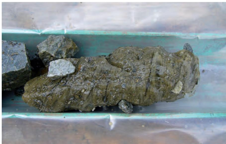
*Figure 3: Frozen core from the drill hole Lazaun I at a depth of 18 to 18.5 m composed of banded ice and debris*
