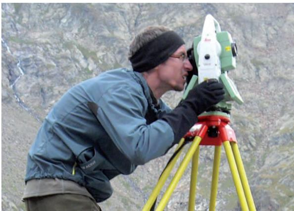
Figure 3: Total Station TCRA 1201 of Leica operated in the field
