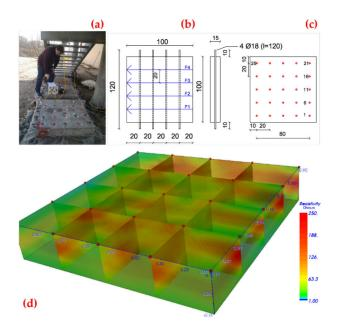
A diffuse increase of the resistivity values due to the curing of the concrete has been detected for the entire volume investigated, except for the lower zones where there is, likely, the accumulation of water (fig. 1d). This is in according with the dielectric permittivity variations showing a negative trend related to the evaporation of the water.
