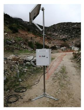
The ERT profile is placed at the base of the tailings dam in order to recognize possible under-seepages that can pollute the groundwater and the surrounding exposed area, with the presence of a city. The system is positioned downstream of two retaining ponds and the aim is to understand whether the variations of water level in the ponds provokes any underseepage.
