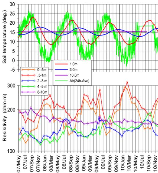
**Fig.5:** Changes of soil temperature at depths of 1, 3, 10 m with daily mean air temperature (upper graph), and changes of analyzed resistivity at five depths up to 10 m near the soil temperature meter (lower graph) since 1 May 2007.
