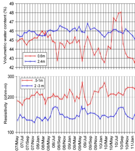
**Fig.6:** Changes of volumetric water content at depths of 0.6m and 2.4 m (upper graph), and changes of temperature-corrected resistivities at depths of 0.5-1 m and 2-3 m (lower graph) since 1 May 2007.
