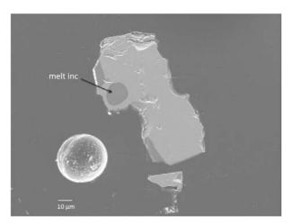
Fig. 2: Titanomagnetite phenocryst containing a silicate melt inclusion from the sample MD-7, Pual Ridge.
