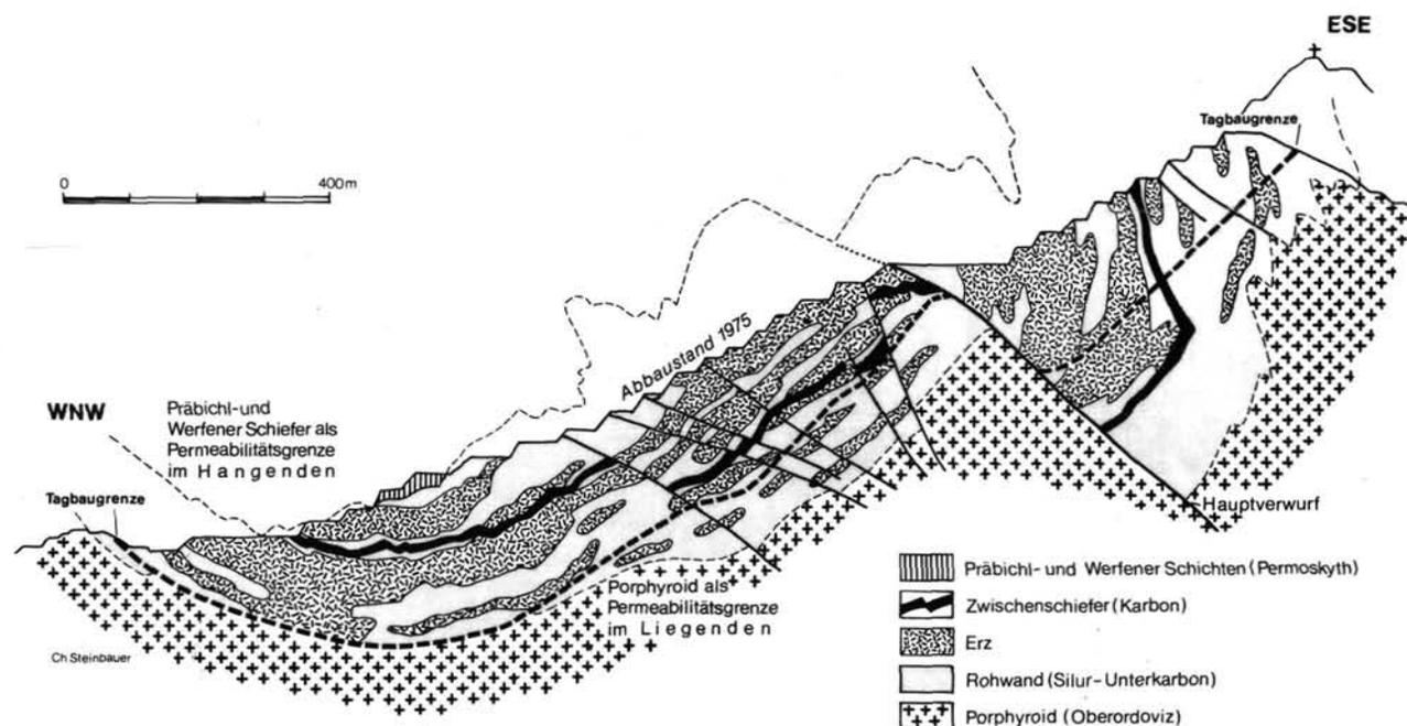
Fig. 4: Cross section through the Erzberg deposit. After Vöest-Alpine Corp.
